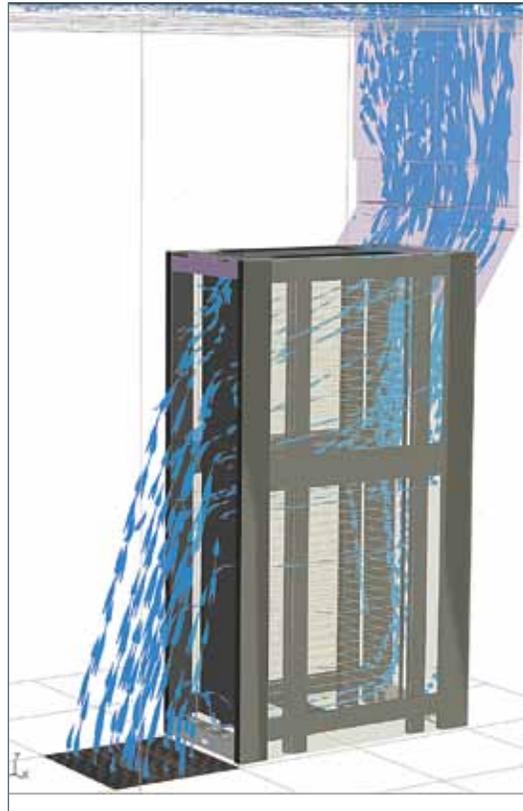
Once containment is in place, the rack becomes an airflow plenum. The data center that invests in containment should not waste the effort by permitting poor rack hygiene and air leakage through the rack (see Figure Five). In an aisle with 10 racks on each side or 20 in the pod, the racks make up approximately 60-percent of the total surface area. Leaking racks could lead hot and cold air to mix, defeating the data center's containment efforts.
