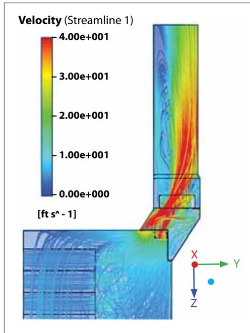
Rack containment eases the containment road map when the chimneys deployed are natively upgradeable in order to add fans. Chimneys address the human factor by removing hot air from the room and the equation (see Figure Six), leaving a cool, comfortable work environment even working up close in front and behind the racks.
